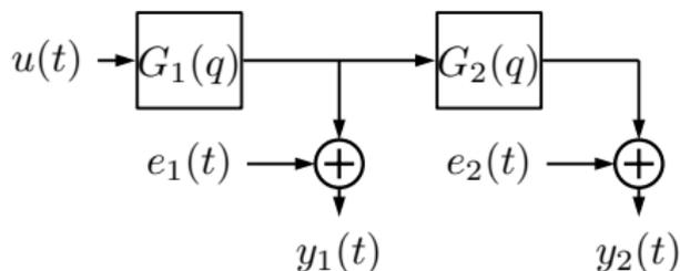
$$\begin{bmatrix} y_1(t) \\ y_2(t) \end{bmatrix} = \begin{bmatrix} \frac{L_1(q, \theta)}{F_1(q, \theta)} \\ \frac{L_2(q, \theta)}{F_2(q, \theta)} \frac{L_1(q, \theta)}{F_1(q, \theta)} \end{bmatrix} u(t) + e(t)$$
